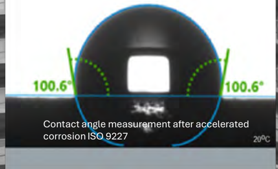
b) Steel with Suststeel system
